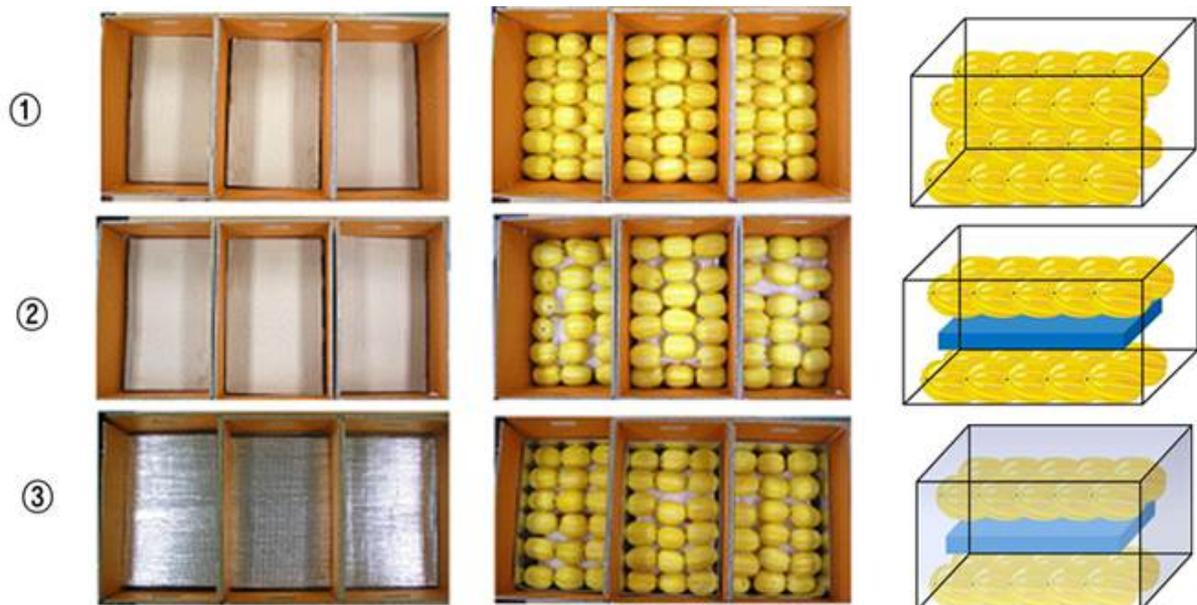
Fig. 1. The storage arrangement of oriental melon packaged in the different treated containers with ① only corrugated box (control), ② corrugated box with ice pack, ③ corrugated box with ice pack and aluminum coated board.
